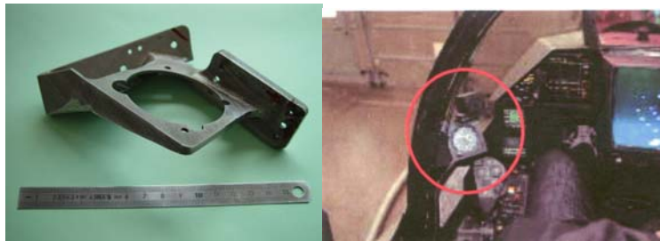
Figure 6: First equipment support made on DM process for Rafale flight tests.
